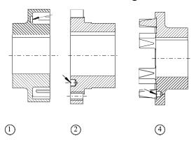
Compensation hole Part 1 of the MAEPEX® Coupling Part 2 of the MAEPEX® Coupling Part 4 of the MAEPEX® Coupling
