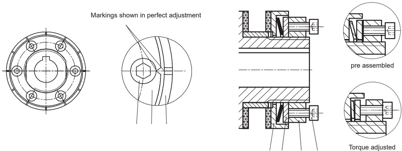
On the face side of the pressure ring (5) and on the outer side of the adjustment nut (2) are markings. These are necessary for the adjustment of the torque as follows. To begin with, the adjustment screws (1) are being screwed out of the nut so far, that they do not stand out.
