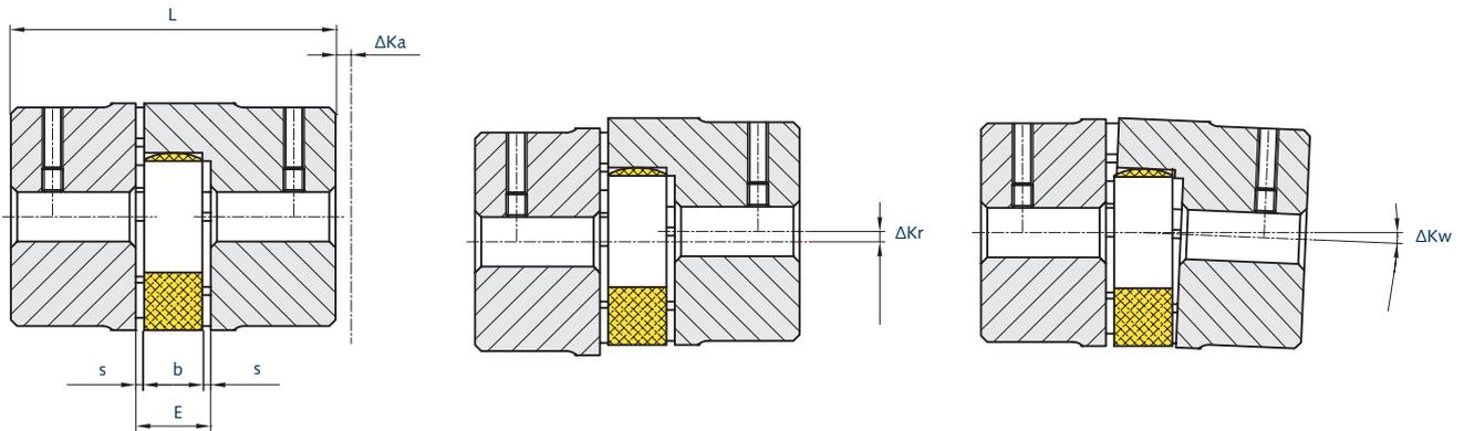
Displacement values for standard couplings (backlash type). The values depend on the speed.
