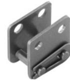
A cranked connecting link **no. 15/C** is needed for uneven attachment configuration **3 x p**. **From 5 x p** its possible to use a straight connecting link no. 11/E.
